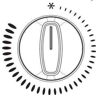
The heat output is controlled by the thermostat. Turn the thermostat knob fully clockwise to maximum setting initially. When the room is warm enough, reduce the setting slowly until the heater just clicks off. The heater will now cycle on and off to maintain your selected room temperature.
